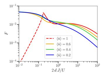
FIG. 2. Control parameter *F* of the theory as defined in (16) plotted as a function of 2dJ/U for different values of the lattice filling. Dashed and solid lines indicate whether the system is in a Mott insulating (only for  $\langle \hat{n} \rangle = 1$ ) or in a superfluid phase, respectively.
